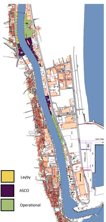
This is the main operational section of the River Port for vessels with draughts less than 6 m. Accessible at the River mouth with a minimum entry width of 61 m, the river bed is dredged to maintain an average depth of 5.7 m. Depths at the berth vary with the majority of operational berths averaging a depth of 5 m or more.
