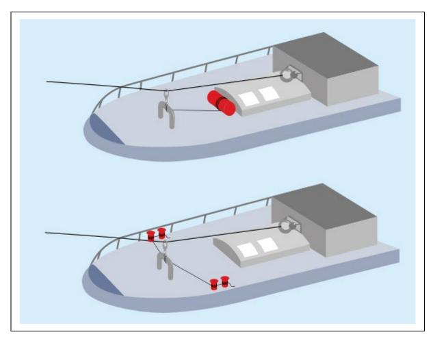
It will be appreciated from the illustration above that a gog rope can limit how far the tug can turn at the end of the towline. In certain circumstances, improper use of a gog rope can severely restrict a tug's manoeuvrability and effectiveness. Therefore, tug operators using a tug to tow conventionally should provide specific training and instruction to the tug master regarding when a gog rope must be used, how it should be made fast, and the effectiveness and limitations of using a gog rope.
