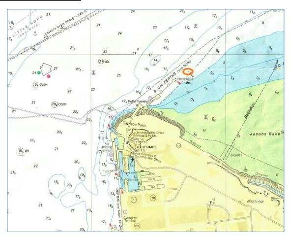
The mooring buoy will be utilised by Ro-Ro vessels berthing on SD.10, when alongside, the ship's mooring lines will create a hazard between the buoy and the vessel. When the berth is not in use the mooring lines will run from the buoy to the berth and be made fast on the downstream dolphin, whilst the ropes are in the water they will be made more conspicuous by coloured marker buoys.
