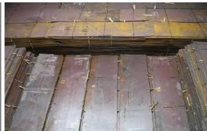
Stow of steel plates in longitudinal and athwartships direction. The upper tiers only are lashed with steel bands.
