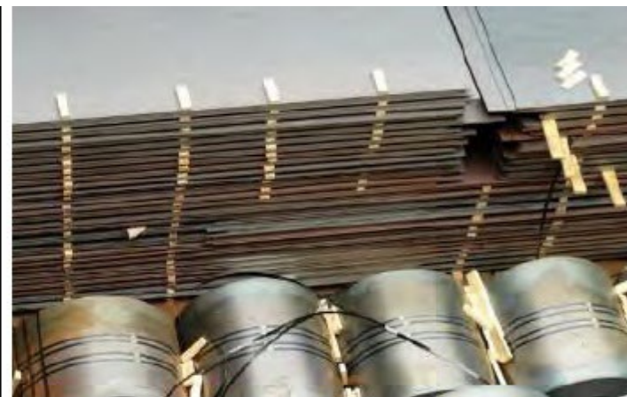
Good application of dunnage for steel plates. It is acceptable to use short hardwood dunnage pieces instead of long bars.
