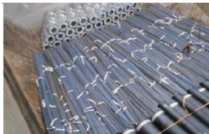
Pre-slung rebar is fanned out in way of the hopper tanks, but sufficient dunnage is placed on the hopper plating to prevent steel-on-steel contact.
