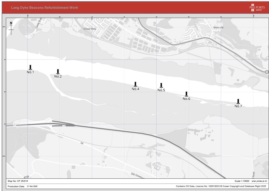
Work to remove marine growth and paint the beacons will be carried out from workboat Tonka. Mariners are requested to navigate this area at appropriate speed to minimise the effects of wash. A listening watch will be maintained on VHF Ch12.
