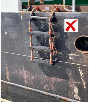
Shackles over side ropes is a commonly seen practice for securing ladders. This is an ineffective and unsafe means of securing the Pilot Ladder. Weight coming on the ladder will result in the shackles bringing up against steps, ferrules/whippings and winnets.
