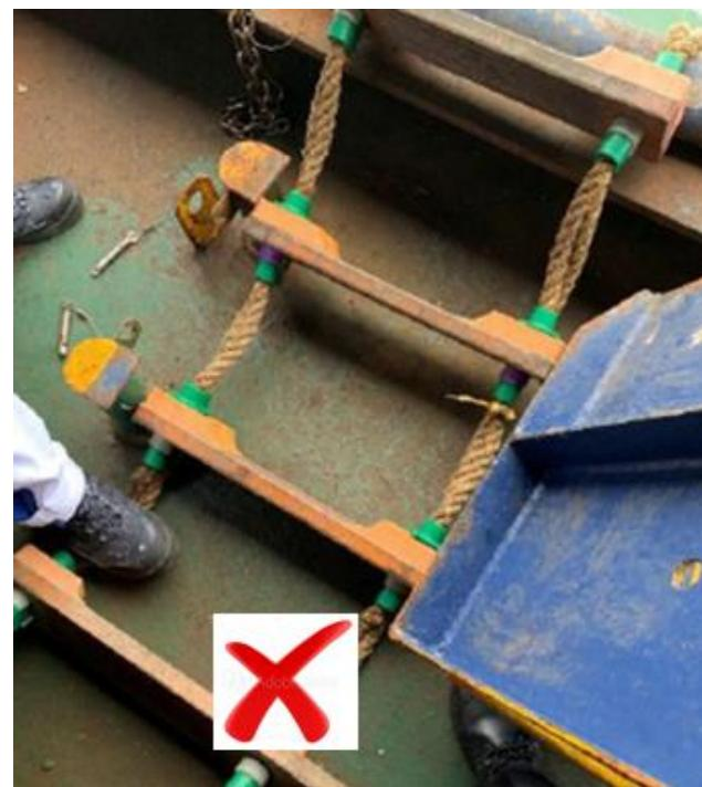
**Embarkation Platform – Trapdoor System. Ladder does not extend 2m above the platform.**
