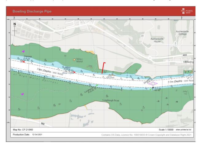
To mark the position of the pipeline, a Special Mark is deployed in position 55°55.766'N 4°30.902'W with the characteristics FI Y 5s.
