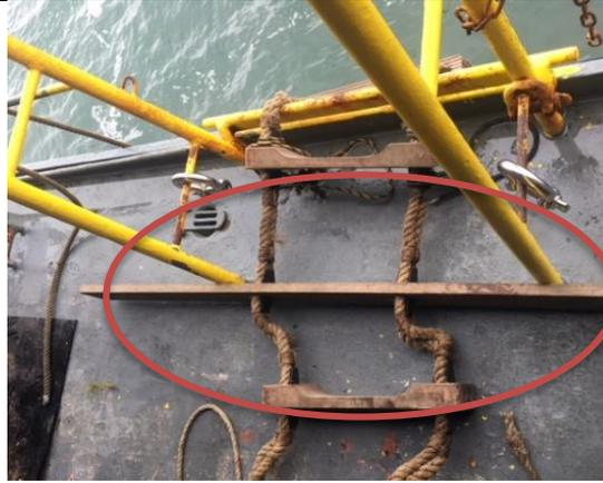
This example shows the completely unacceptable practice of bracing a spreader against the stanchion of the handrail.
