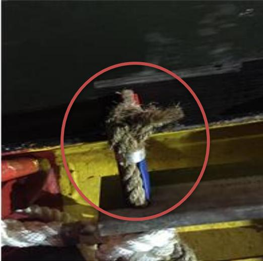
This example shows a poorly maintained pilot ladder.
