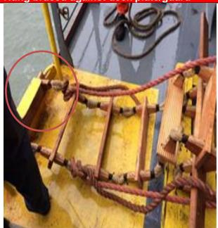
This example shows a rung braced against a "deck plate/guard". There is evidence of the side ropes being secured by extra lines, but these lines are unbalanced and slack.
