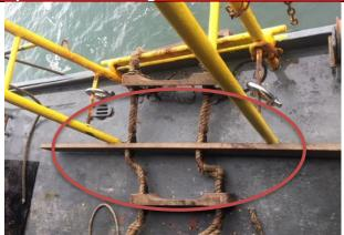
This example shows the completely unacceptable practice of bracing a spreader against the stanchion of the handrail.
