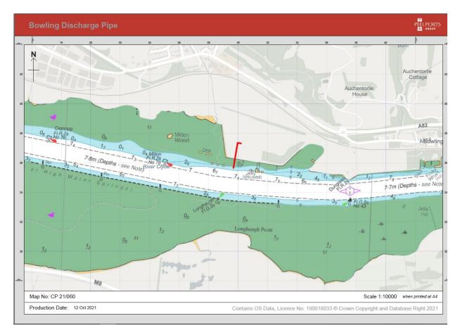
To mark the position of the pipeline, a Special Mark is deployed in position  $55^{\circ}55.766'N$  4°30.902'W with the characteristics Fl Y 5s.
