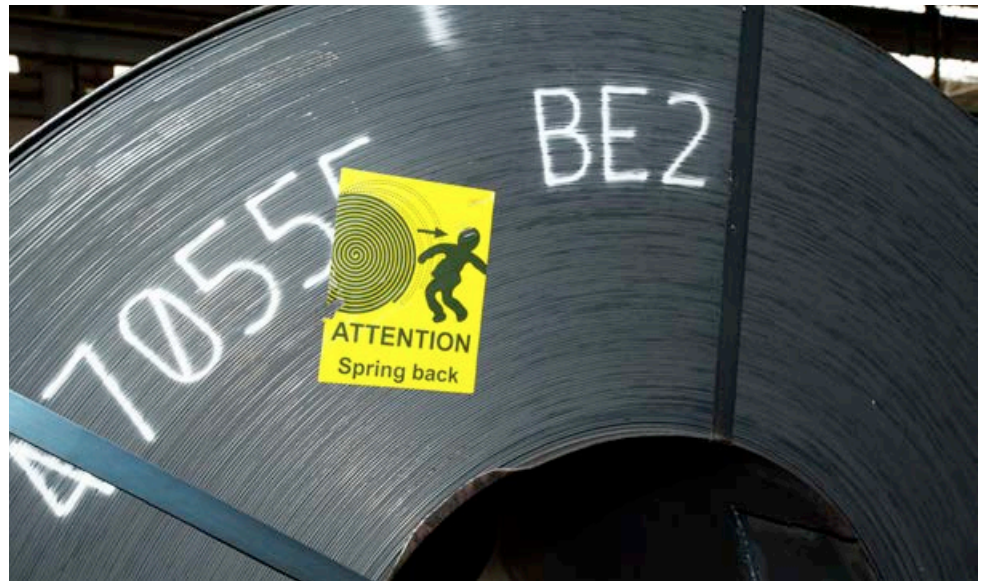
Photograph 21 Banding strip on broad coil with warning sticker of 'spring-back' risks
