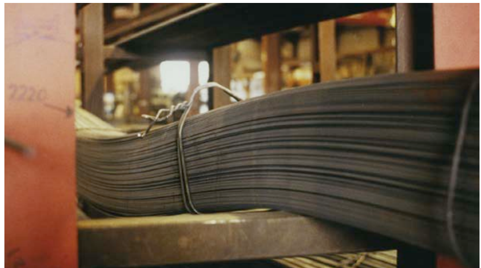
Photograph 22 Damaged banding wire suggests that it was being used to lift the bundle
