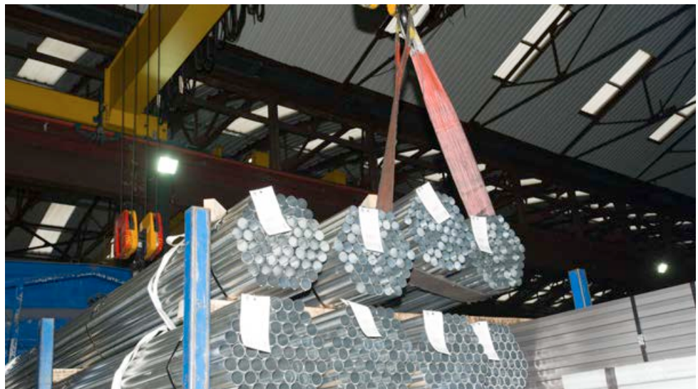
Photograph 34 Web sling lifting long tube product using twin hoist crane.
