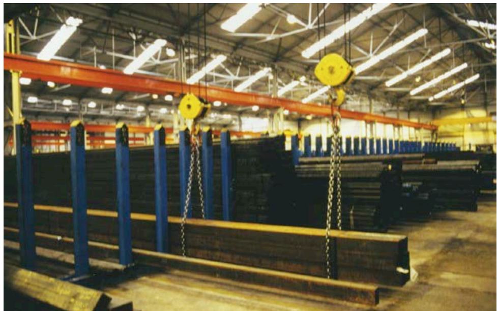
Photograph 25 Use of twin hoist crane for lifting long product. Each hoist is operated independently and remotely
