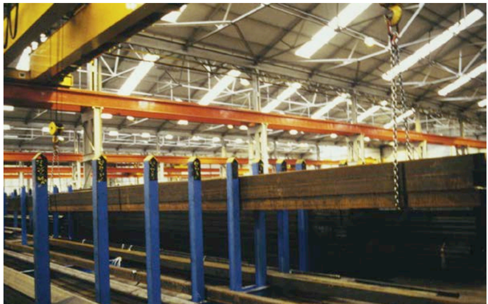
Photograph 27 Hoists linked together to effect horizontal lift out of racking. Crane operator is at a safe distance in a protected gangway throughout
