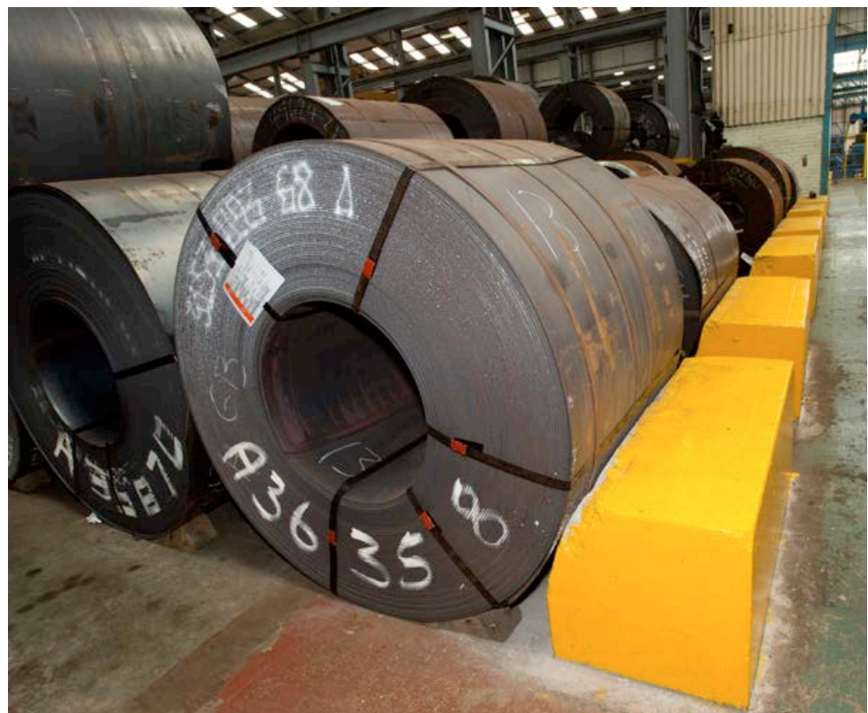
Photograph 7 Substantial concrete barriers, with reinforcing bars sunk into the floor, for containing broad coils
