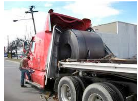
Photograph 59 The result of an inadequately restrained coil combined with hard braking
