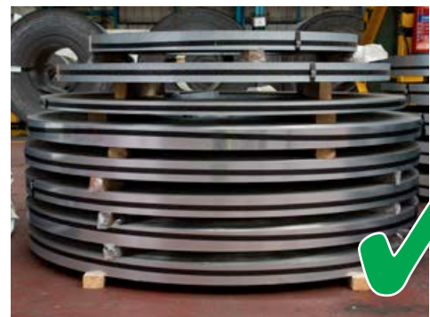
Photograph 6 The same coils but stacked safely with largest diameter at the bottom and smallest diameter at the top
