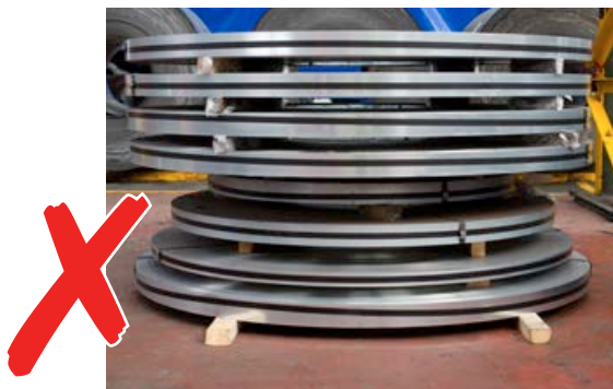
Photograph 5 A stack of coils which are unsuitably stacked presenting instability
