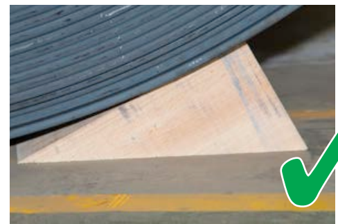
Photograph 11 The chock is placed correctly with the longest edge on the floor
