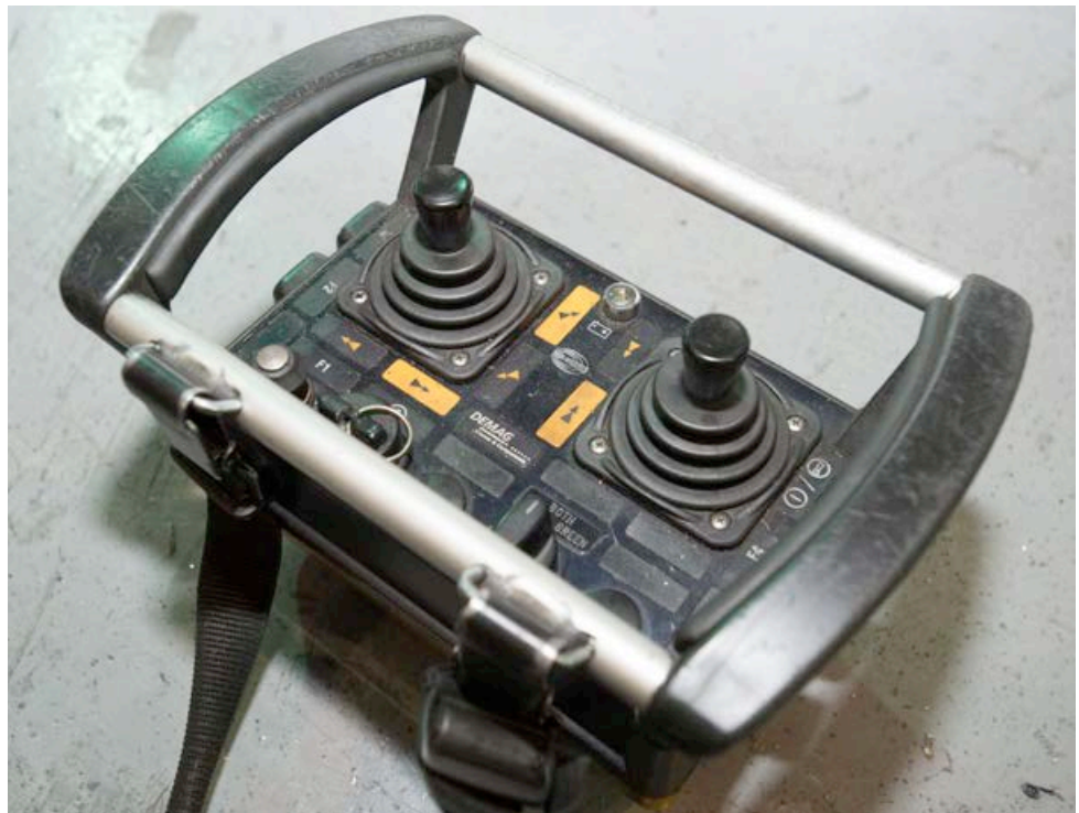
Photograph 30 Harness type remote control in clean condition with suitable directional labelling
