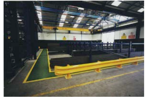
Photograph 2 Good layout of rack storage with clearly defined pedestrian routes and separation from fork-lift trucks
