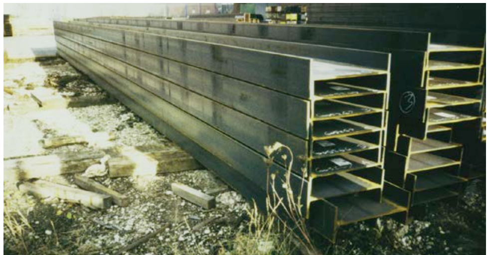
Photograph 3 Free-standing stacks of broad, long product on firm, level ground using wooden bearers. Note poor control of tripping hazards in access area
