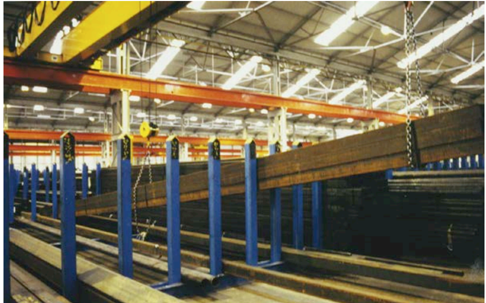
Photograph 26 Load is inclined by outermost hoist. Inner hoist's lifting chain is moved towards the opposite end
