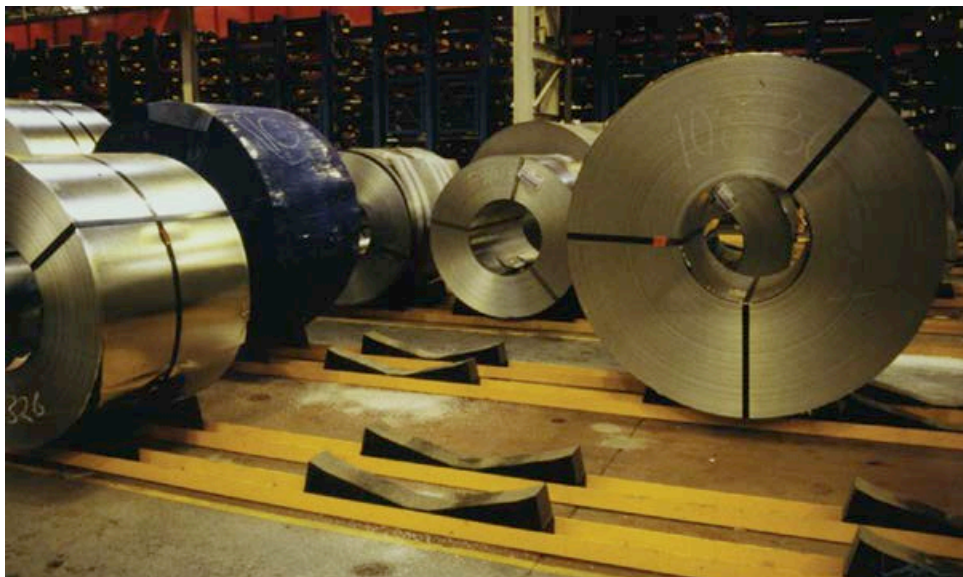
Photograph 13 Broad coil storage in plastic coil supports on floor-mounted inverted metal channels
