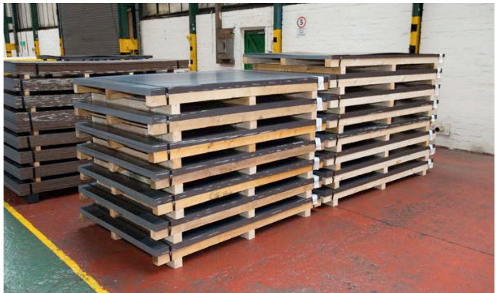
Photograph 18 Sheet/plate banded onto pallets with minimal exposed sharp edges
