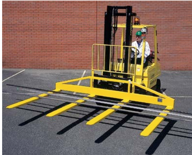
Photograph 36 Fork lift truck fitted with four-fork attachment. These can be used for carrying long, narrow product or plate/sheet
