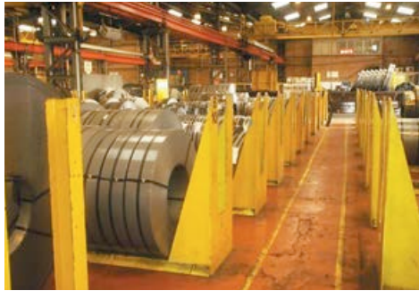
Photograph 1 Storage of narrow coils in standing coil rack. Good stock containment with safe access for slingers and a protected/clearly defined pedestrian route
