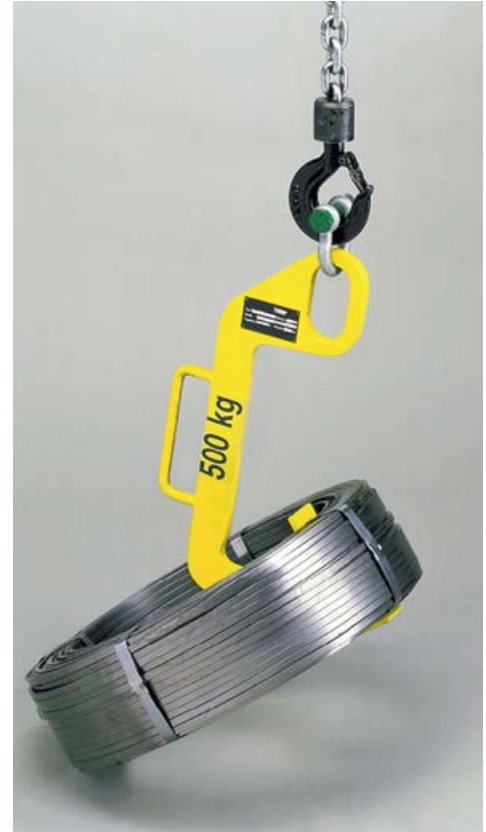
Photograph 43 Turning C-hook which enables coils which are lying flat to be lifted to the vertical plane.
