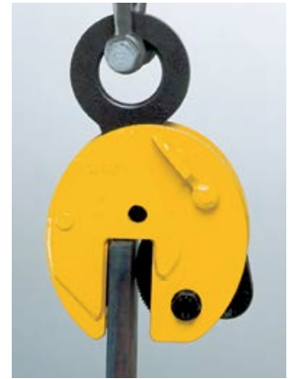
Photograph 49 Vertical plate clamp in use
