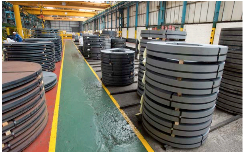
Photograph 4 Free-standing stacks of narrow coils (bore-vertical) on suitable bearers on a solid floor. Individual coils are separated by bearers for safe/easier attachment of coil lifters or other handling equipment. The banding ensures the coil is maintained in shape.
