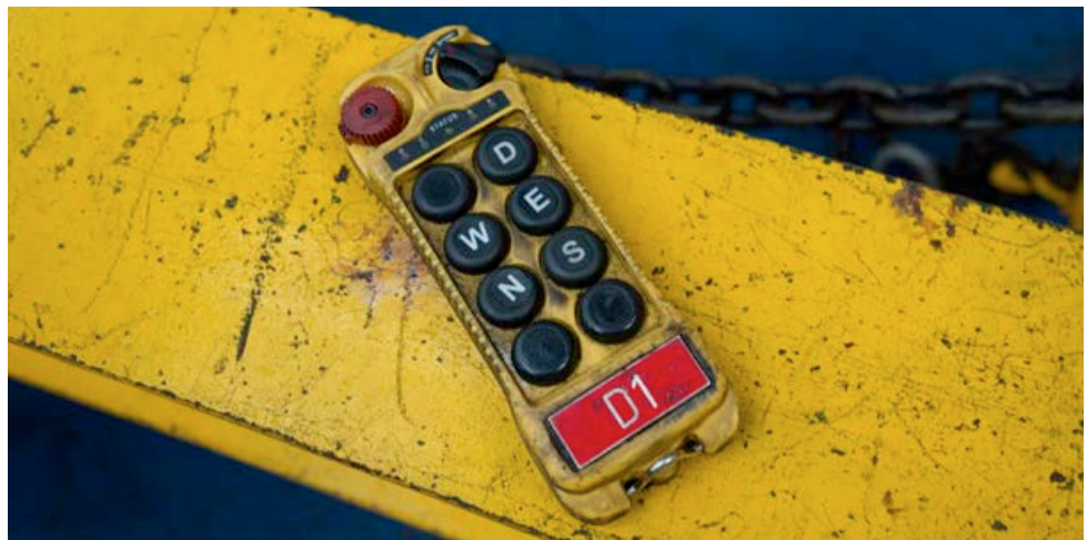
Photograph 29 Remote control for overhead crane in general good condition but with some worn labelling of control buttons
