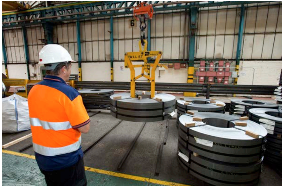
Photograph 47 Horizontal coil lifter raising narrow, bore-vertical coil
