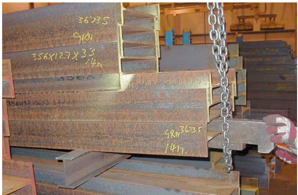
Photograph 40 Using a fish plate to lift long broad product
