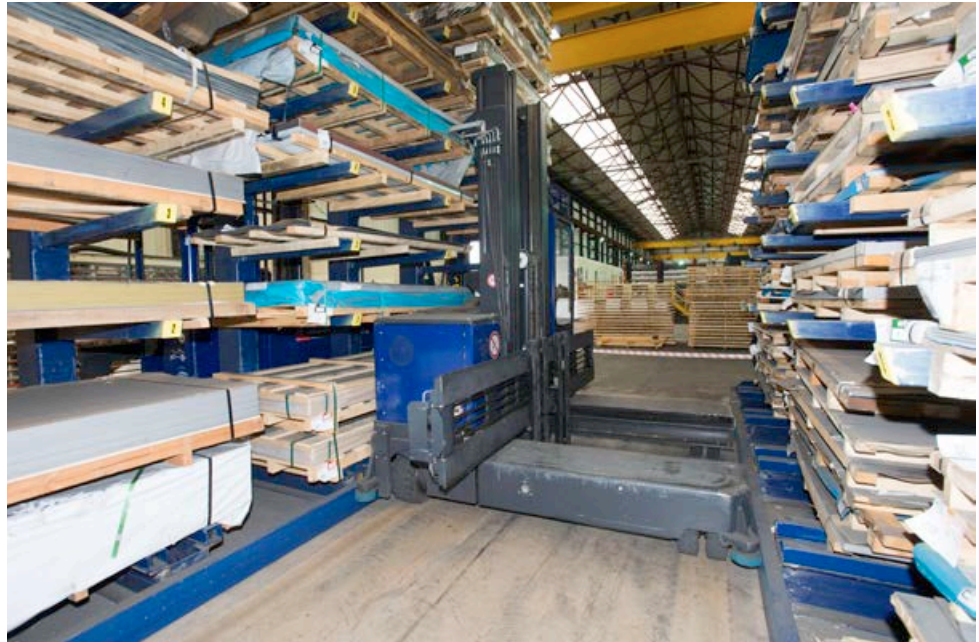
Photograph 57 Guided aisle specialist reach truck for cantilever racking system
