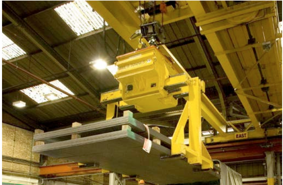
Photograph 52 Telescopic dog lifting equipment
