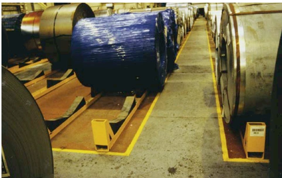
Photograph 14 Broad coil storage using floor-mounted inverted metal channels Containment posts fitted to channel ends and clearly defined working areas and pedestrian routes
