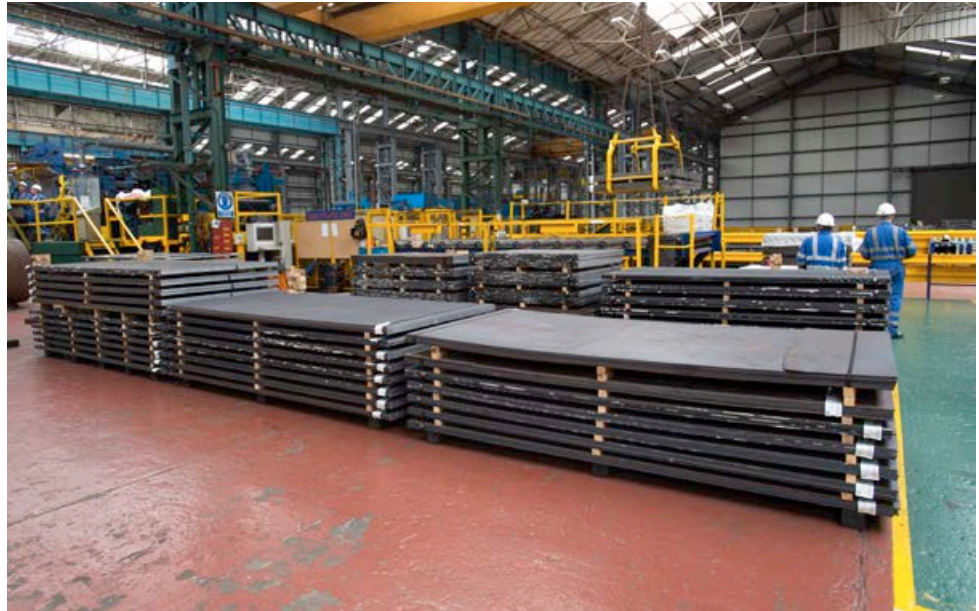
Photograph 17 Tidy and well-spaced, free-standing floor storage of plate; separation of small quantities of sheet by suitable bearers (battens)
