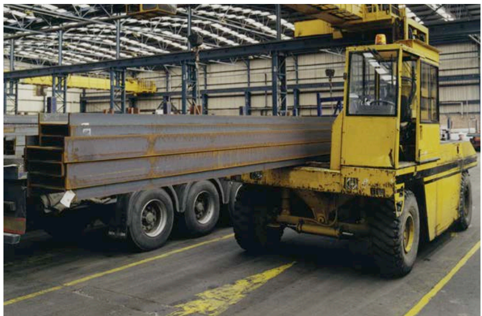
Photograph 56 Use of a side-loader lift truck for handling long, broad product
