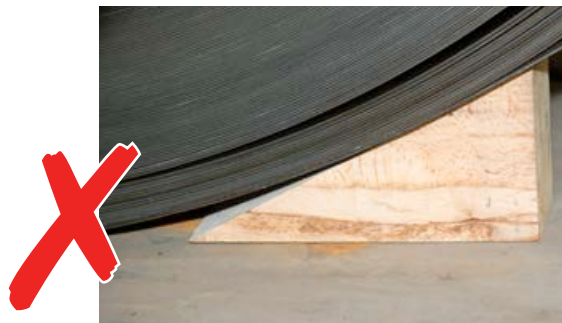
Photograph 10 The chock is placed incorrectly with the longest edge against the coil
