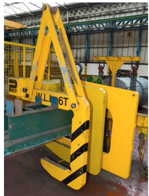
Photograph 44 Storage beams for C-hooks
