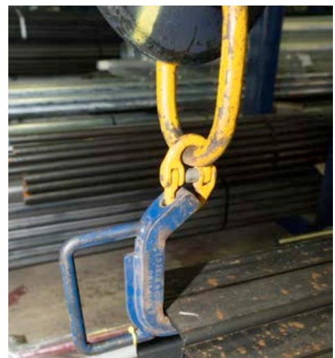
Photograph 41 Using a splitter bar to allow safe positioning of bearers and attachment of lifting accessories
