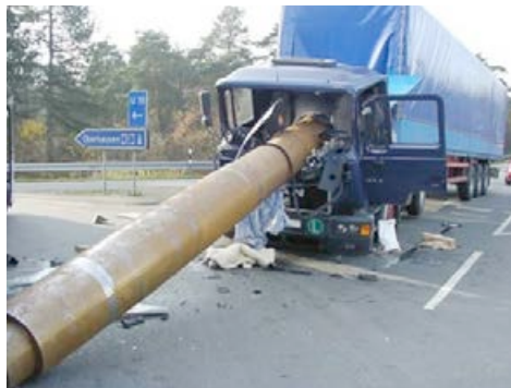
Photograph 58 Accident showing what can happen when a load is unsecured
