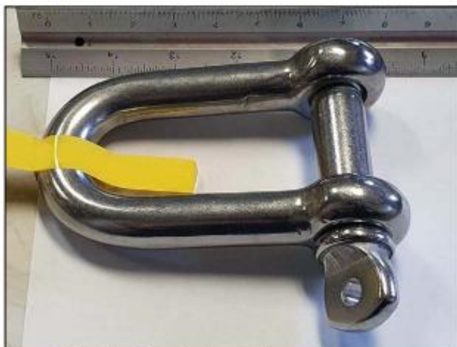
Figure 1: Steel shackle used as heaving line weight
