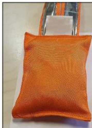
Figure 2: Bean bag supplied by tug company as a safe alternative heaving line weight
